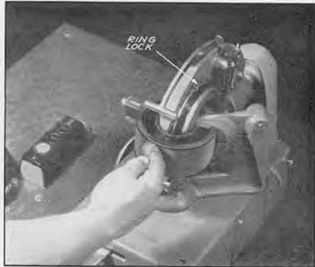
(Above) FIGURE 3. Magazine ring being loaded with wire prior to actual winding.
