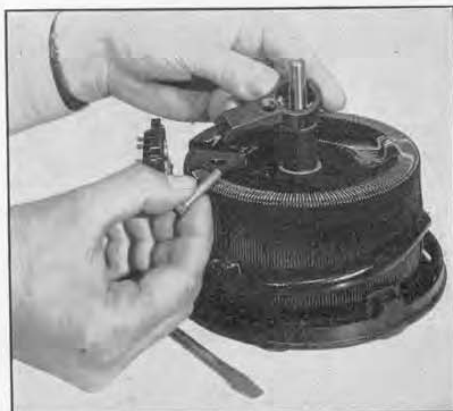
(Above) FIGURE 6. The coil is firmly held to the base by the coil clamp here shown during installation.
