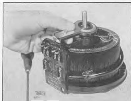
(Below) FIGURE 7. Installing the brush take-off sub-assembly which carries brush current from radiator to terminal, supports the upper end of the terminal strip and serves as a resilient brush stop.
